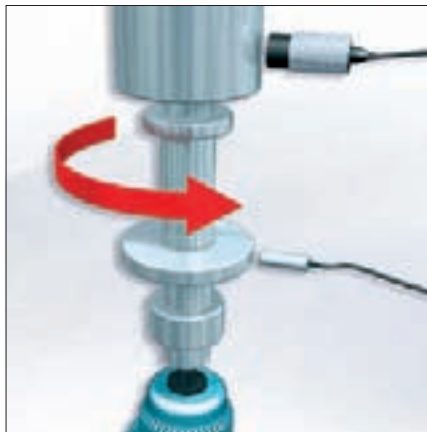
Eccentricity control of a rotating shaft
