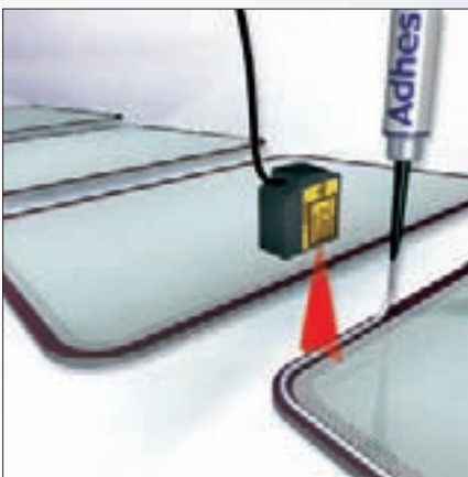
Glue seam inspection
