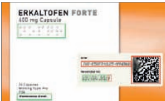
Date/Batch code verification (OCR/OCV)
