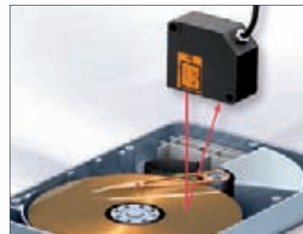
Disk surface inspection
