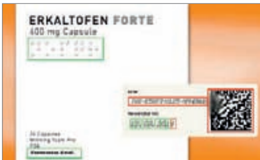
Date/Batch code verification (OCR/OCV)
